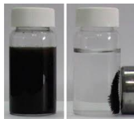
Figure 1. Image of a solution containing the magnetic graphene-based nanocomposite.
